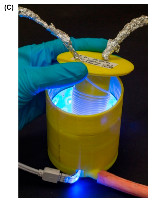
Figure 1. Schematic representation of the microflow setups for (A) gas-liquid trifluoromethylation and (B) perfluoroalkylation of cysteine. (C) Picture of the photomicroreactor (more details regarding the setup can be found in the Supporting Information).
